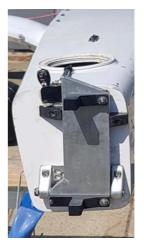
Any attachment to the actual hull whose only use is to anchor control systems or to strengthen the stern in a particular area is not considered part of the rudder assembly and is to be include in the overall hull length. Rule D.4.1(a).
