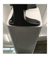
Attachments to the hull whose only purpose is to restrict the sideways movement of the gudgeon are allowed, however in this case the outside block is flush with the side of the hull and would not be allowed under Rule E.5(c).
