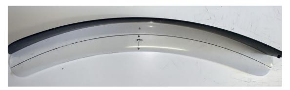
Lay trailing edge of dagger board on drawn line, start with middle of board and middle of template lining up.
