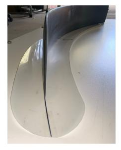
If trailing edge meets line on all points or drawn line is visable on inside edge of both ends on dagger board minimum radius of 1190mm is met.
