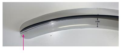
If drawn line is visable on outside edge of dagger board minimum radius of 1190mm is **NOT** met and board is illegal.
